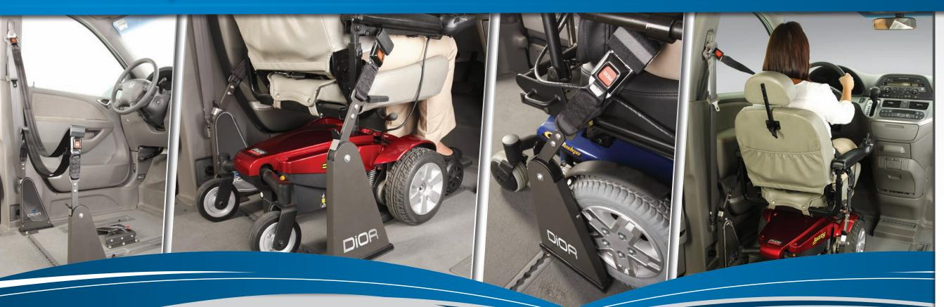
In seconds, the innovative DiOR and QLK docking system puts you exactly where you need to be. DiOR's pivoting arms move forward as you enter, providing you with the right lap belt angles that other systems can only approximate. Meanwhile,
