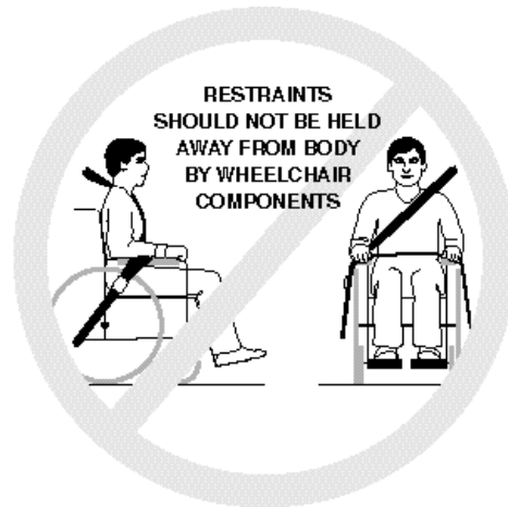
Figure 8 - Restraints should not be held away from the body by wheelchair components or parts, such as the wheelchair armrests or wheels.
