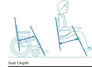
The seat depth is increased even more when a chair is equipped with legrests that have calf supports. Calf supports hold the legs forward of the front edge of the seat. If this is not taken into consideration when ordering the wheelchair, this may prevent you from positioning your buttocks against the backrest and would then cause you to sit in a slumped sitting posture.
