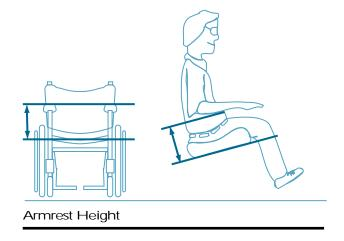
The armrest height of a wheelchair with a fixed-height armrest is given as a single value. For wheelchairs with adjustable-height armrests, a range of heights is given. Some adjustable armrests have infinite adjustments within the range, while others have a limited number of preset height adjustments.
