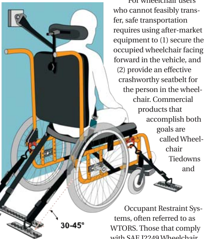
This wheelchair is secured by a four-point tie-down with occupant using a three-point belt restraint.
